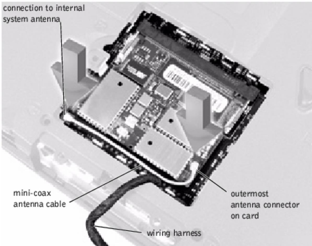
➔ **NOTICE:** If a wireless network adapter card contains two mini-coax antenna connectors, connect the mini-coax cable to the outermost antenna connector as shown.
