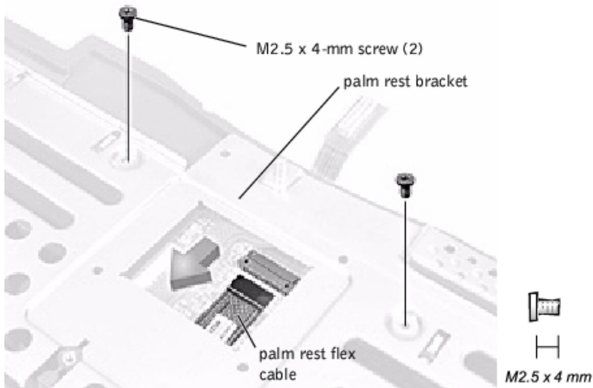
7. Remove the two M2.5 x 4-mm screws securing the palm rest bracket.
