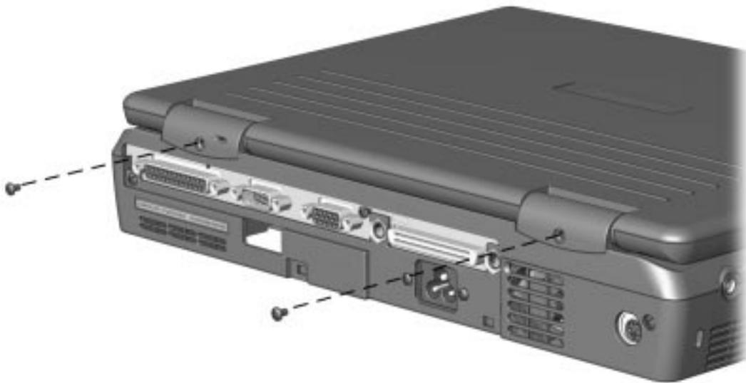
*Figure 5-21. Removing the Hinge Cover Screws*
