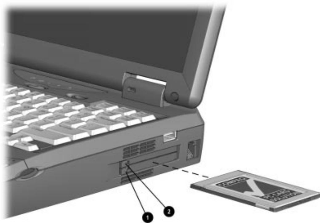
*Figure 5-4. Removing the PC Card*
