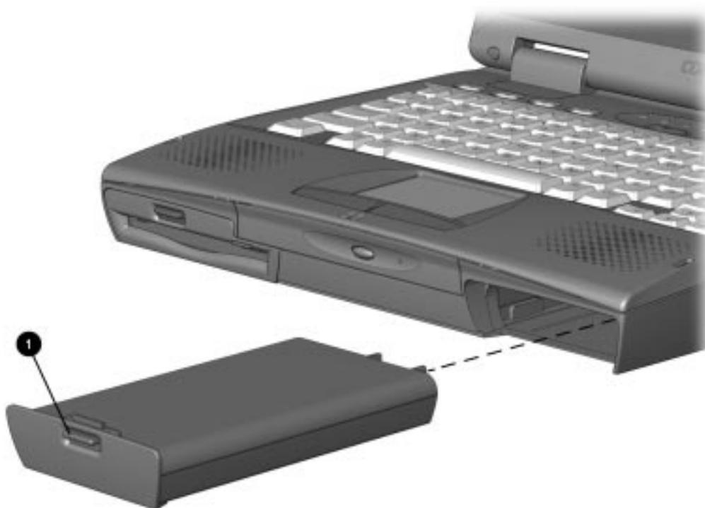
*Figure 5-2. Removing the Battery Pack*
