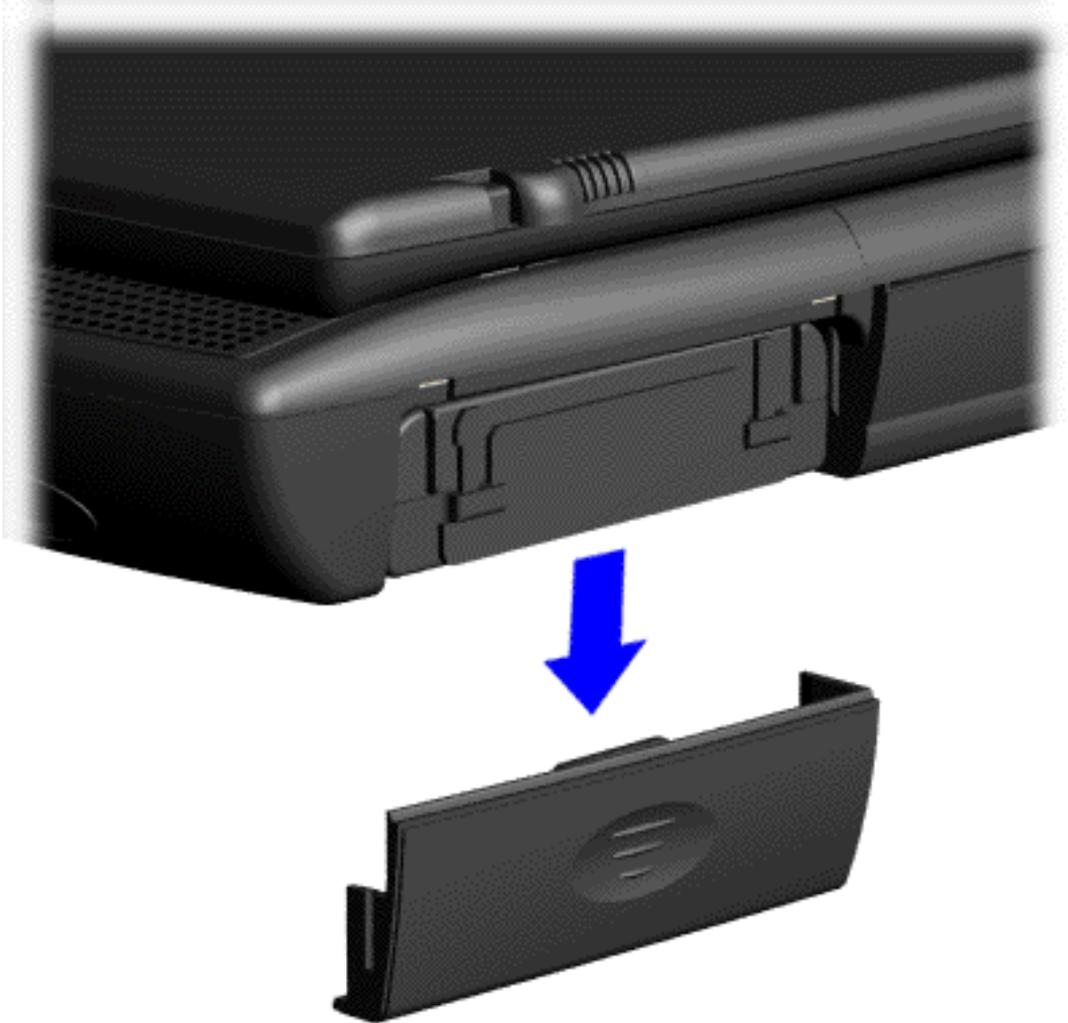
To remove the battery pack, complete the following steps:
