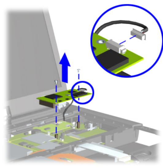
Removing the Network Interface Card
