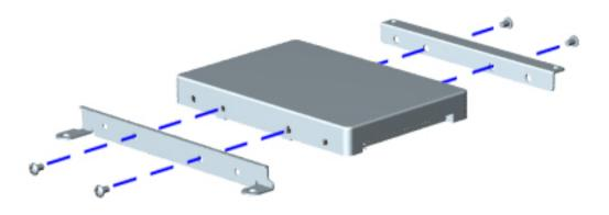
Removing the Hard Drive Mounting Brackets, continued
