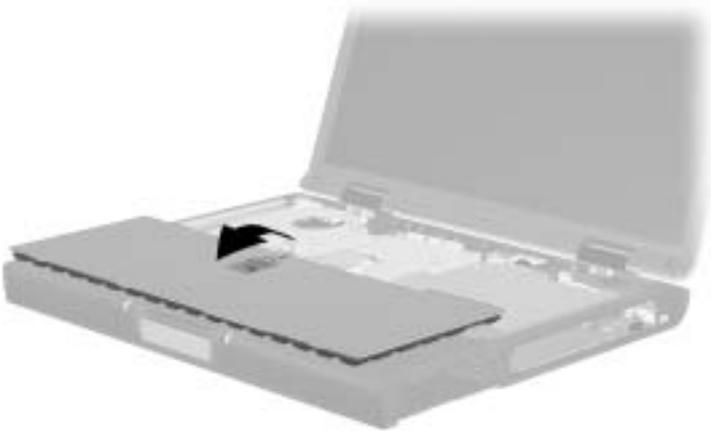
***Figure 5-18. Releasing the Keyboard***
