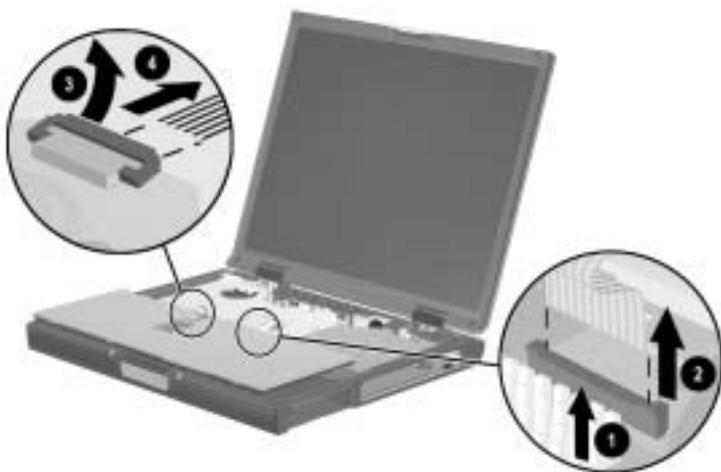
**Figure 5-19. Disconnecting the Keyboard-to-TouchPad Cable**
