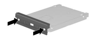
Figure C-2. PM1.5  $\times$  3.5 Screw Location
