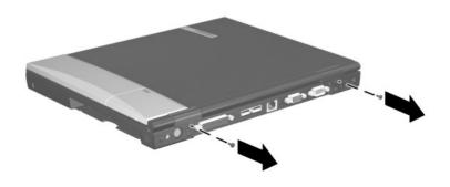
Figure 5-16. Removing the Switch Cover Screws
