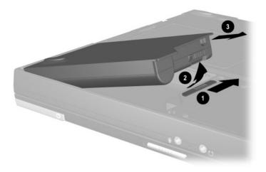
Figure 5-2. Removing the Battery Pack
