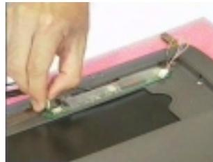
6. Remove the two screws as shown below.
