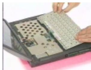
3. Disconnect the keyboard cable from the main board.
