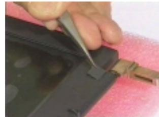
5. Remove the five screws from the LCD module.
