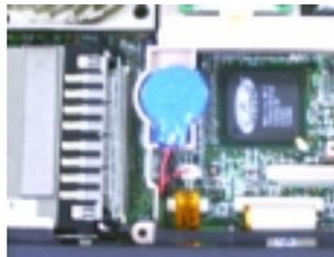
4. Remove the RTC battery.
