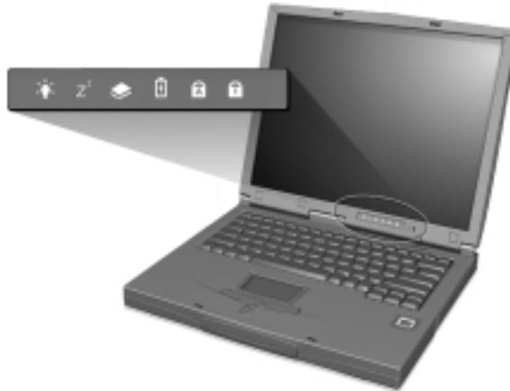
The Power and Standby status icons are visible even when you close the display cover so you can see the status of the computer while the cover is closed.
