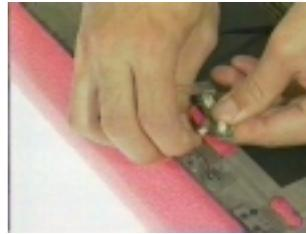
7. Disconnect the inverter to led cable, and speaker to led cable.
