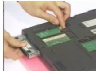
**WARNING:** Be careful not to break the FDD FPC cable, when sliding out the module.
