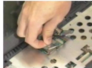
5. Release the two screws on the main unit.
