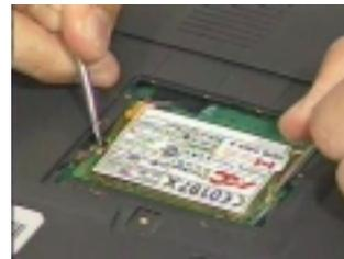
3. Remove the modem board from the main board.
