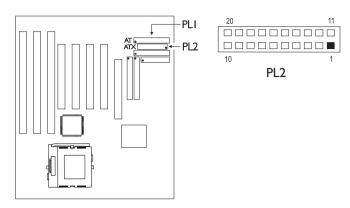
The pin assignment of the ATX power connector is shown below.
