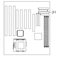
pin I of the drive edge connector(s). The end-most connector should be attached to the drive you want to designate as Drive A.
