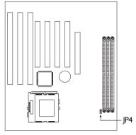
compatibility problems with PC SDRAM DIMMs or you are using EDO/SDRAM DIMMs, set the SDRAM clock according to the AGP clock (1-2 On).
