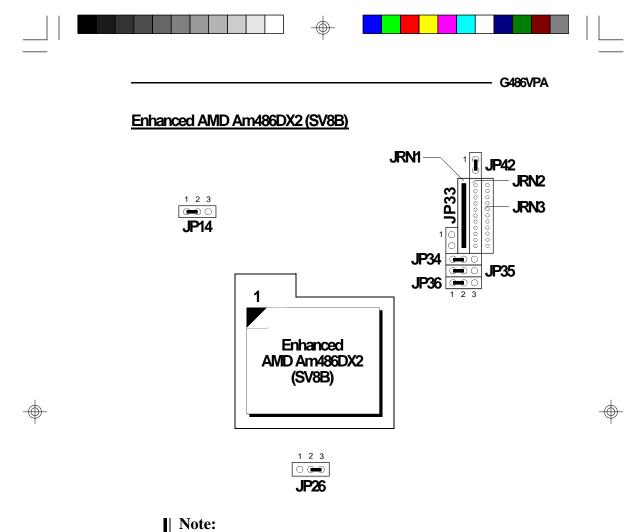
Note: Jumper JP42 is used to support Enhanced Am486DX2 CPUs (starting with Revision A of the system board).
