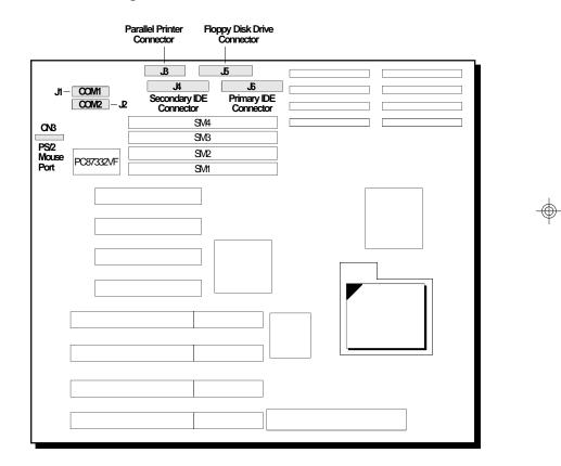
Locations of the Built-in Ports on the System Board
