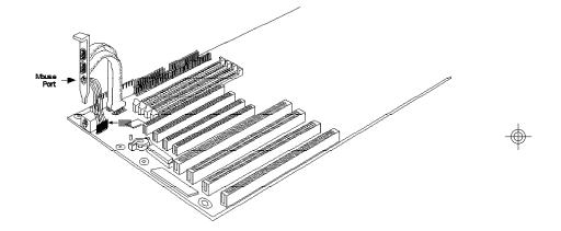
The PS/2 Mouse Port on the G486VPA System Board
