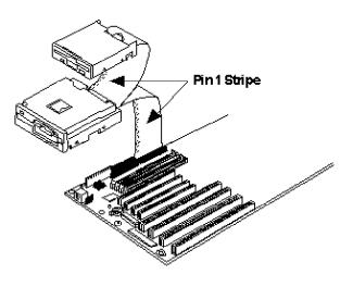
The Floppy Disk Connector on the G486VPA System Board
