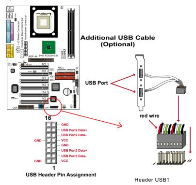
When plugging the USB cable into Header USB1, users must make sure the red wire is connected to the first pin.
