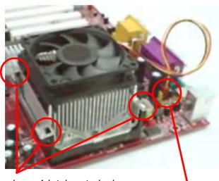
Press down 4 latches to lock fan to fan socket
