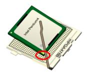
Make sure that all CPU pins have completely entered the socket and then lower down the lever to lock up CPU to socket.
