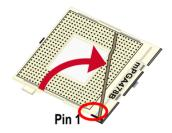
Configure Pin 1 of CPU to Pin 1
