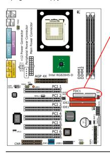
Floppy Disk Drive Connector: Orient the red line on the floppy ribbon cable to Pin1.
