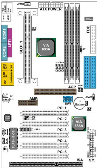
NOTE: FOR 100 / 133MHz CPU ENVIRONMENT, THE SDRAM MUST COMPLY WITH PC-100 / PC-133 SPEC.
