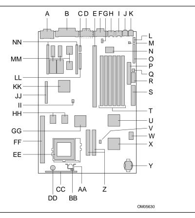
Figure 1. Motherboard Components
