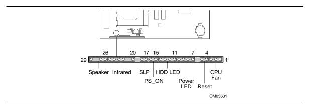
Figure 4. Front Panel I/O Connectors
