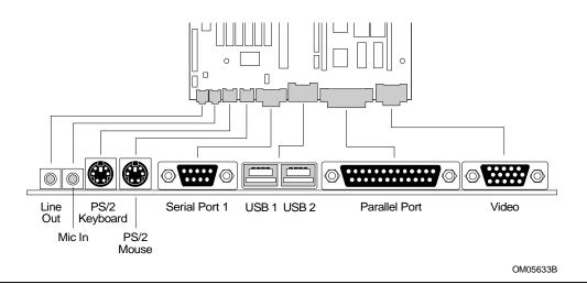
Figure 5. Back Panel I/O Connectors
