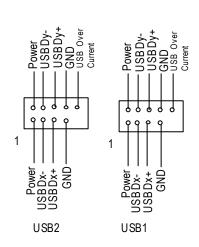
Be careful with the polarity of the front panel USB connector. Check the pin assignment while you connect the front panel USB cable. Please contact your nearest dealer for optional front panel USB cable.
