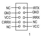
Make sure the pin 1 on the IR device is aling with pin one the connector. To enable the IR/CIR function on the board, you are required to purchase an option IR/ CIR module. For detail information please contact y our autherized Giga-Byte distributor.
