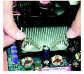
Fasten the heatsink supporting-base onto the CPU socket on the mainboard.
