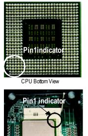
Locate Pin 1 in the socket and look for a (golden) cut edge on the CPU upper corner. Then insert the CPU into the socket.
