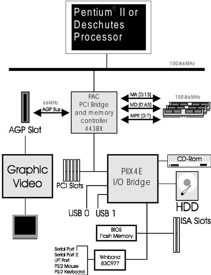
Figure 5: System Block Diagram
