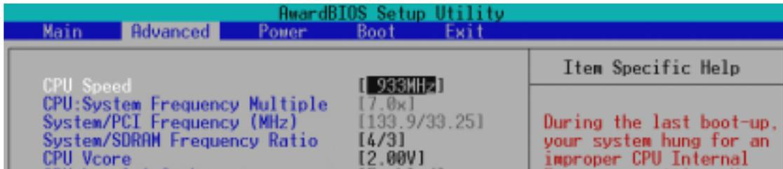
**Cause for Hangup: Improper CPU Speed**
