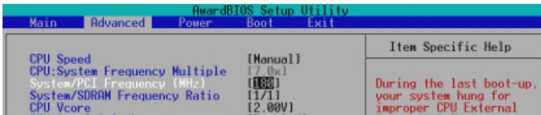
**Cause for Hangup: Improper System/SDRAM Frequency Ratio**
