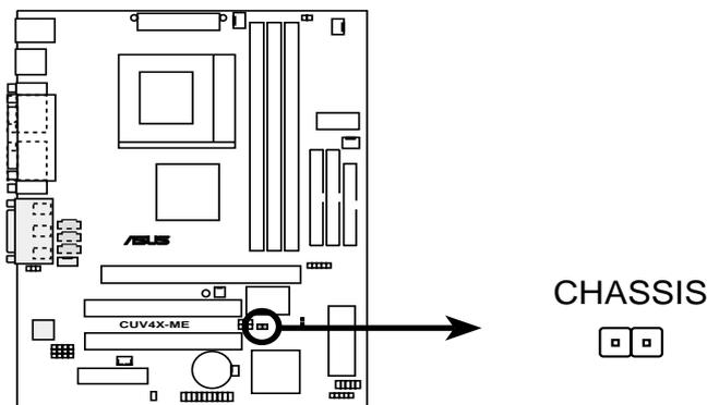
CUV4X-ME Chassis Open Alarm Lead
