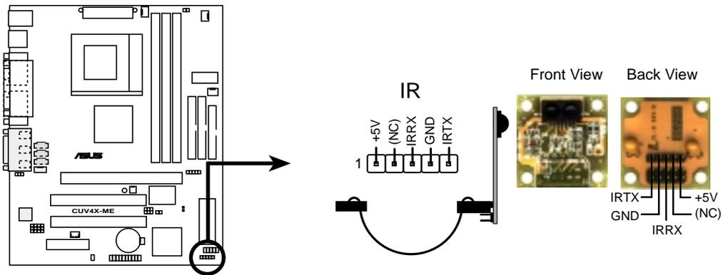
**CUV4X-ME Infrared Module Connector**
