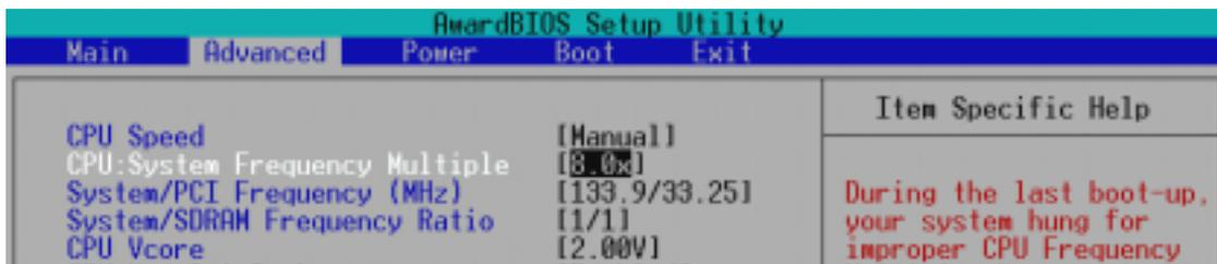
**Cause for Hangup: Improper CPU: System Frequency Multiple
