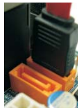
Connect the SATA data cable to one of the orange eSATAII connector (eSATAII_BOTTOM (Port5))
