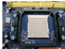
STEP 1: Lift Up The Socket Lever
