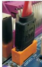
Connect the SATA data cable to the eSATAII connector (eSATAII_TOP)
