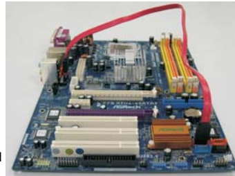
Connect the SATA data cable to the red eSATAII connector (eSATAII_BOTTOM)
