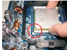
STEP 2 / STEP 3: Match The CPU Golden Triangle To The Socket Corner
