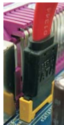
Connect the SATA data cable to the eSATAII connector (eSATAII_TOP)
