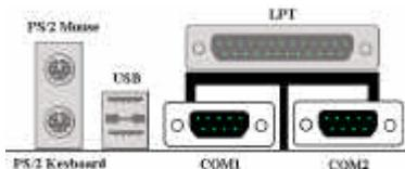
This motherboard provides two COM ports, you can connect an external modem, mouse or other devices that support this communication protocol.
