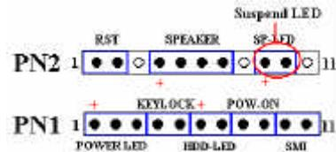
Insert the two-threaded suspend LED cable into pin 9 and pin 10. If you install it in the wrong direction, the LED light will not illuminate correctly.
