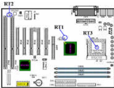
The Thermistors RT1 and RT3 are already onboard, RT1 (or R317) is used to detect the system environment temperature, and RT3 is used to detect the CPU temperature. The RT2 is for you to connect an additional thermistor to detect the temperature in the location of your choice. You can buy the thermistor at an electronics store, and ask for a 10K $\Omega$  thermistor which should be OK. Please don't use too long of a lead wire for the thermistor.
