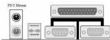
Attach a PS/2 mouse to this 6-pin Din-connector.
