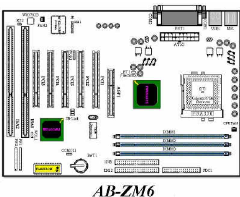
Figure 1-2. Motherboard component location
