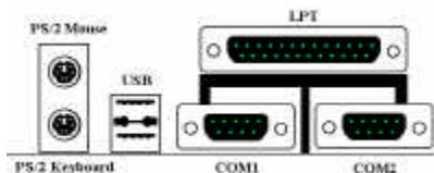
Figure 2-10. ZM6 back panel connectors
