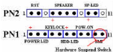
Attach the cable from the case's front panel suspend switch (if there is one) to this header. Use this switch to enable/disable the power management function by hardware.
