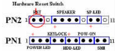
Attach the cable from the case's front panel Reset switch to this header. Press and hold the reset button for at least one second to reset the system.
