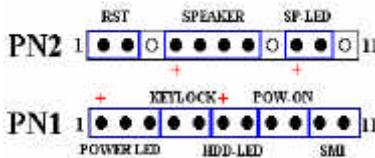
Figure 2-9. The definition of PN1 and PN2 pins
