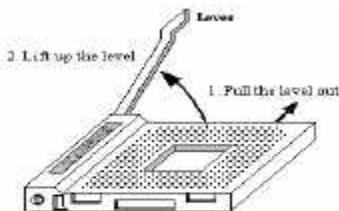
Figure 2-3. Socket 370 and open its lever
