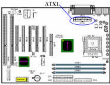
Attach the connector from the power supply to the ATX1 connector here. Remember you have to push the connector from the ATX power supply firmly to the end with the ATX1 connector, insuring that you have a good connection.
