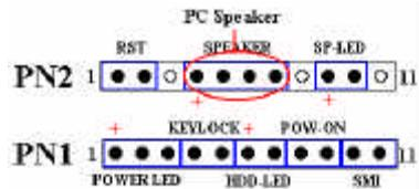
Attach the cable from the system speaker to this header.
