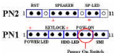
Attach the cable from the case's front panel power switch to this header.
