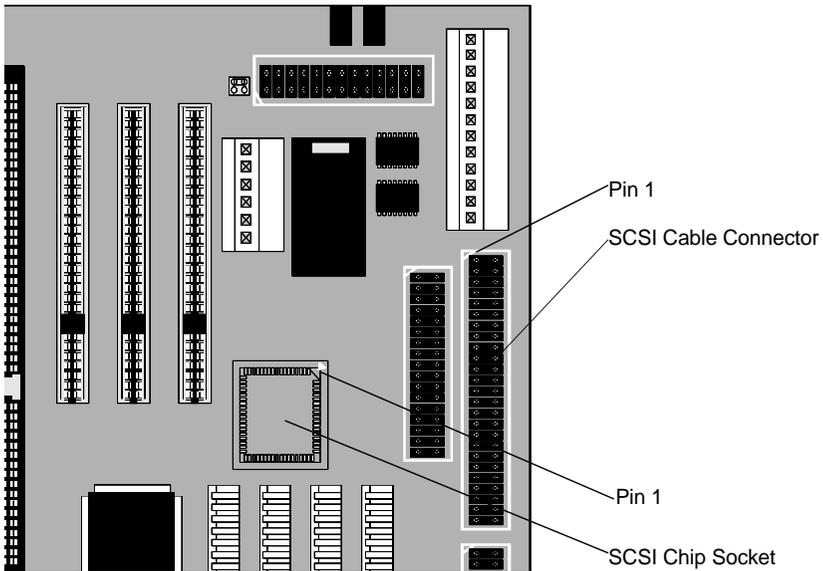
4. Locate the SCSI host adapter socket on the mainboard and identify the pin 1 (beveled) corner of the socket.
