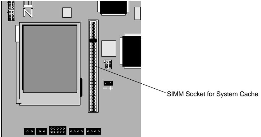
3. If you are upgrading your system cache memory, remove the SIMM you are replacing by gently pulling the SIMM out of the socket.
