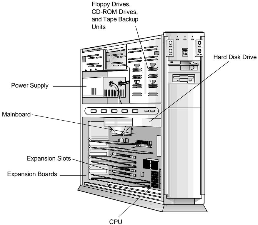
Vertical systems have all the same components as desktop systems. The figure shows the mainboard and common components inside a vertical system unit case.
