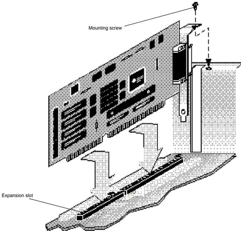
6. Slide the new board into place. Press firmly so the edge connector on the card slides all the way into the expansion slot.
