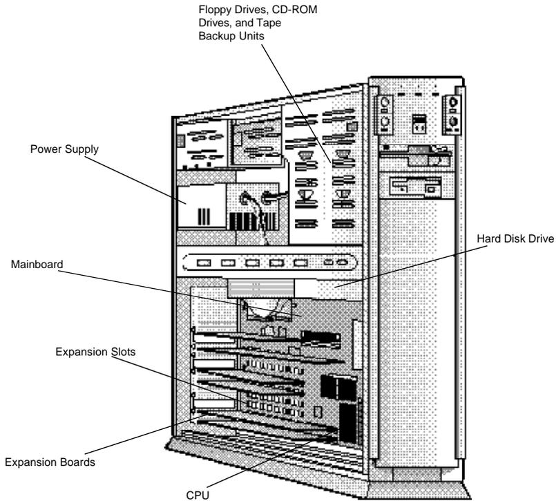
Vertical systems have all the same components as desktop systems. The figure shows the mainboard and common components inside a vertical system unit case.
