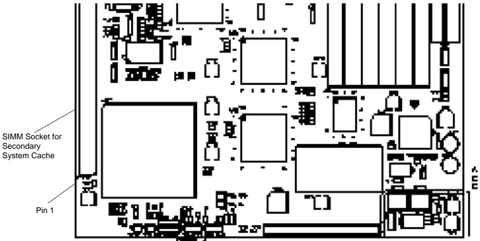
3. If you are upgrading your system cache memory, remove the SIMM you are replacing by gently pulling the SIMM out of the socket.
