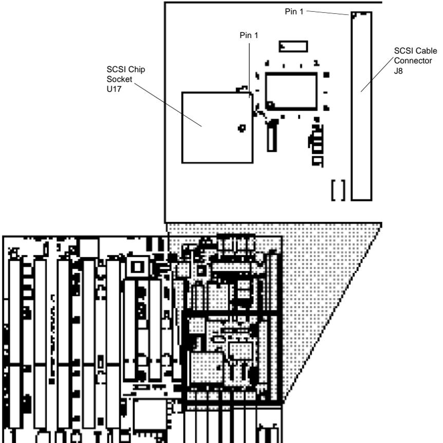
4. Locate the SCSI host adapter socket on the mainboard and identify the pin 1 (beveled) corner of the socket. If you need help finding the SCSI host adapter socket, see the figure above.
