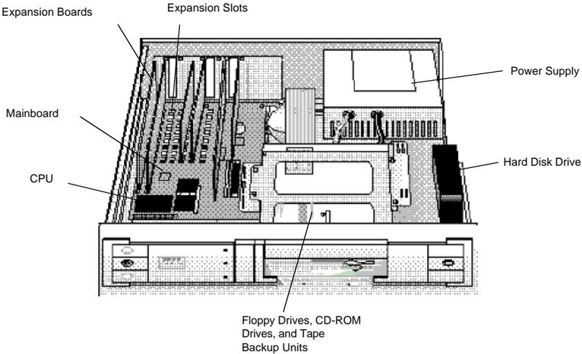
The mainboard is the large circuit board at the bottom of the system unit case. It is the heart of your system. All of the other components inside the case work for the mainboard. The power supply delivers electricity to the mainboard. The disk drives, keyboard connectors, and other parts of the system unit bring information to and from the mainboard.
