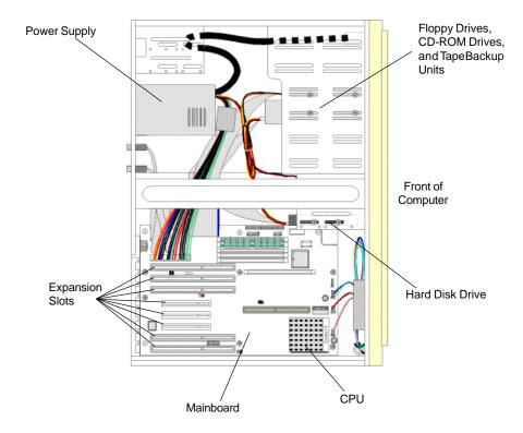
Tower systems have the same components as desktop systems. The figure above shows the mainboard and typical components inside a Tower case.
