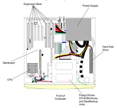
The mainboard is the large circuit board at the bottom of the chassis. It is the heart of your system. All of the other components inside the case work for the mainboard. The power supply delivers electricity to the mainboard. The disk drives, keyboard connectors, and other parts of the system unit bring information to and from the mainboard.
