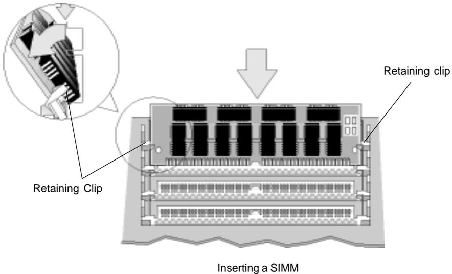
5. Ensure the SIMM seats correctly. If not, remove and repeat Step 4.
