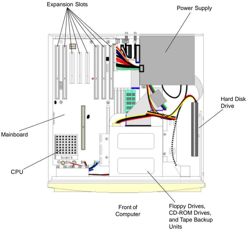
The mainboard is the large circuit board at the bottom of the chassis. It is the heart of your system. All of the other components inside the case work for the mainboard. The power supply delivers electricity to the mainboard. The disk drives, keyboard connectors, and other parts of the system unit bring information to and from the mainboard.
