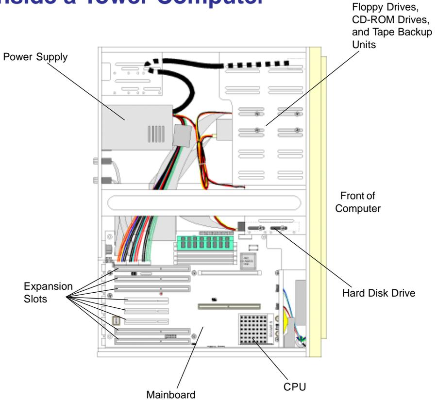
Tower systems have the same components as desktop systems. The figure above shows the mainboard and typical components inside a Tower case.
