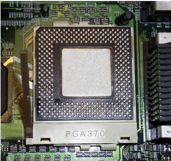
Pin 1 on the CPU is denoted by a small dot on one of the corners and Pin 1 on the ZIF socket is denoted by an angled corner. Never force a CPU into a socket. Forcing a CPU to seat will bend the pins on the CPU and possibly damage the motherboard. Check with your vendor or manufacturer for proper voltage selection.
