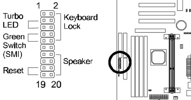
**Pins [3 & 5] Turbo LED switch** - The Turbo function is not supported by this mainboard. Therefore, the Turbo LED will always remain lit as long as the system power is on.
