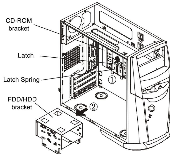
In order to remove the FDD/HDD bracket, ① lift the latch of the latch spring with one hand and ② remove the FDD/HDD bracket with the other hand.
