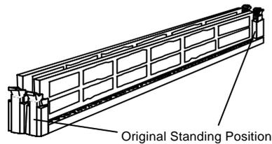
check if the clip is properly locked onto the hollow of the DIM module. If not, press slightly to lock it.
