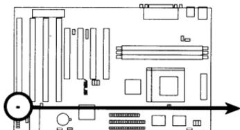
TIP: If the case-mounted LED does not light, try reversing the 2-pin plug.
