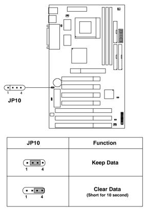
**Note:** You can clear CMOS by shorting 3-4 pin for 10 second, while the system is off. Then, return to 2-3 pin position. To be able to clear the CMOS, There is always a 3V Standby power, so you need to unplug the system.
