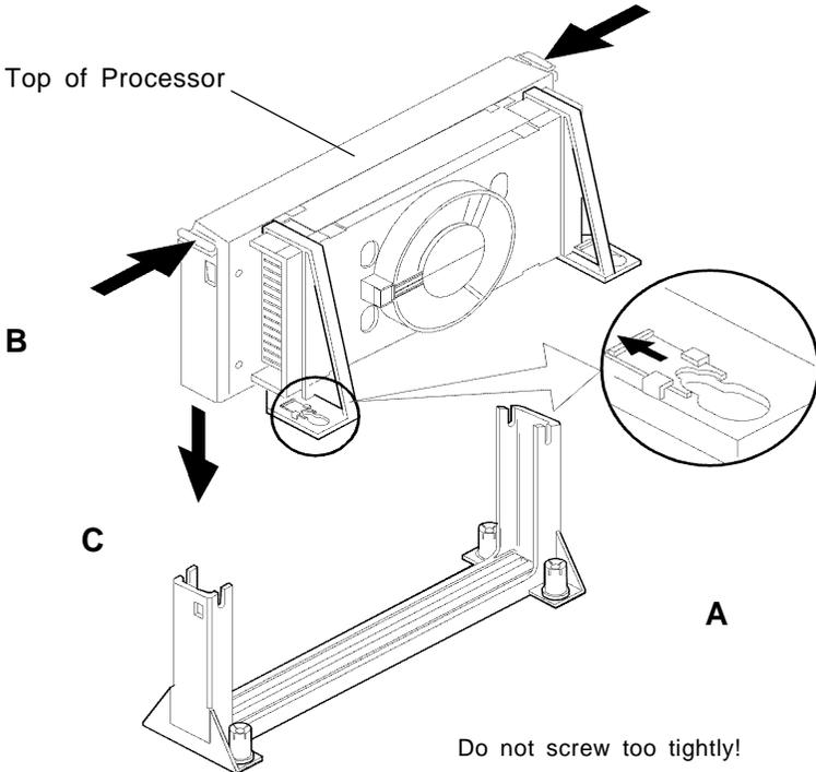
6. Slide the clips on the supports (A) forward until they click into place to hold the pegs securely. Apply slight pressure on the peg and push the peg toward the clip while pushing the clip forward. Push the latches on the processor (B) outward until they click into place in the retention mechanism. The latches must be secured for proper electrical connection of the processor.
