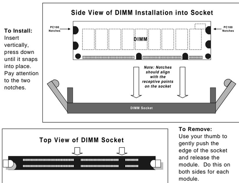
Figure 2-1. Installing the DIMM
