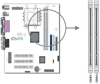
Your board comes with two DIMM sockets, providing support for up to 1GB of main memory using unbuffered and registered DIMM modules from 8MB to 512MB. On this motherboard, DRAM speed can be set independent from the CPU front side bus speed. Depending on the DRAM clock speed setting in the BIOS setup (Chapter 3), appropriate memory modules must be used. For 66MHz DRAM speed, use PC66 memory; for 100MHz DRAM speed, use PC100 memory; for 133MHz DRAM speed, use PC133 memory.
