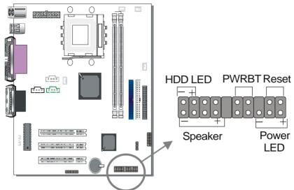
Plug the computer case's front panel devices to the corresponding headers on the Motherboard.
