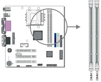
Your board comes with two DIMM sockets, providing support for up to 1GB of main memory using unbuffered DIMM modules from 32MB to 512MB. On this motherboard, DRAM speed can be set independent from the CPU front side bus speed. Depending on the DRAM clock speed setting in the BIOS setup (Chapter 3), appropriate memory modules must be used. For 100MHz DRAM speed, use PC100 memory; for 133MHz DRAM speed, use PC133 memory.
