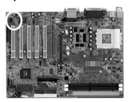
The SPDIF-in/out connector supports the digital audio. This connector must be connected to the cable from an external device. (Ex. 2-channel decoded AC-3 from DVD decoders)
