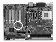
If you want to use a USB keyboard, you must enable the onchip USB & USB keyboard support function in BIOS's Integrated Peripherals menu (See Section 3-4). USB is an open industry standard, providing a simple and inexpensive way to connect up to 125 devices to a single computer port. Keyboards, mice, tablets, digitizers, scanners, bar-code readers, modems, printers and many more can all be used at the same time.
