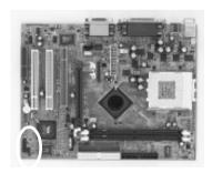
If you enable the UART 2 Mode in BIOS's Integrated Peripherals menu the COM2 port will support IR functions. (See section 3-4)
