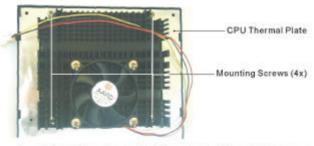
Heat Sink & Fan Assembly Mounted on Xeon™ Processor
