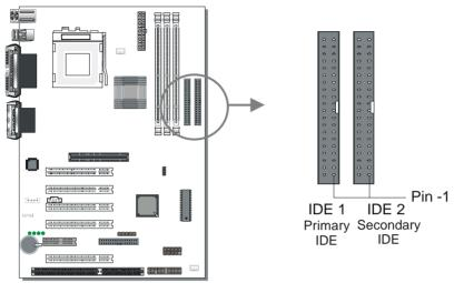
This Motherboard offers two primary and secondary IDE device connectors (IDE1, IDE2). It can support up to four high-speed Ultra DMA 33/66HDD or CD-ROM.
