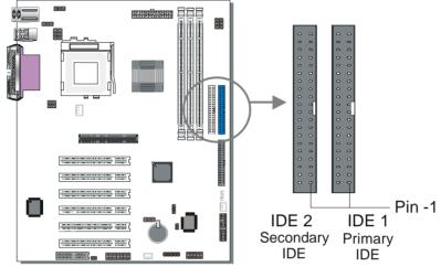
This Motherboard offers two IDE device connectors, a primary (IDE1) and a secondary (IDE2). It can support up to four high-speed HDD or CD-ROM.
