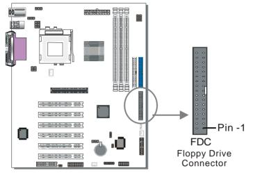
The system supports 5 possible floppy drive types: 720 KB, 1.2 MB, 1.44 MB, 2.88 MB, and LS-120. In addition, this Motherboard supports a 3-mode (720KB/1.2MB/1.44MB) floppy commonly used in Japan. Connect one side of the 34-pin flat cable to the floppy drive and plug the other end to the floppy drive connector on the Motherboard. This Motherboard can support up to 2 floppy drives.
