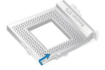
2. Align the blunt edge of the CPU with the matching pinhole distinctive edge on the socket.
