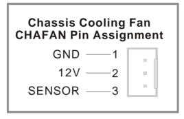
*Note: CPU cooling fan must be installed to prevent CPU from overheating and ensure system stability. Chassis cooling fan is optional, depending on whether there is cooling fan in your chassis.*
