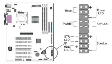
Plug the computer case's front panel devices to the corresponding headers on the Motherboard.
