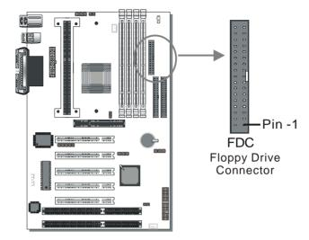
The system supports 5 possible floppy drive types: 720 KB, 1.2 MB, 1.44 MB, 2.88 MB, and LS-120. In addition, this Motherboard supports a 3-mode (720KB/1.2MB/1.44MB) floppy commonly used in Japan. Connect one side of the 34-pin flat cable to the floppy drive and plug the other end to the floppy drive connector on the Motherboard. This Motherboard can support up to 2 floppy drives.
