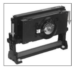
4. After completely inserting the CPU, push the two locks on top of the CPU outward. Now your CPU is ready for use.
