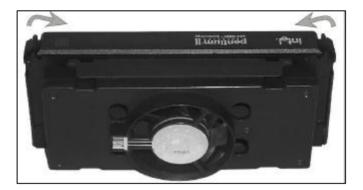
Insert the CPU into the retention module. The CPU fits in the CPU slot in only ONE way, do not try to force it in.
