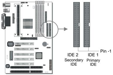
This Motherboard offers two primary and secondary IDE device connectors (IDE1, IDE2). It can support up to four high-speed Ultra DMA 33HDD or CD-ROM.
