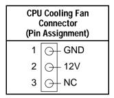
Note: Make sure the pin assignment of our CPU Cooling Fan is matched with this connector before connecting it, otherwise, you may damage either the mainboard or the cooling fan.
