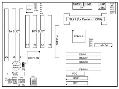
Figure 1–2. Mainboard Default Setting
