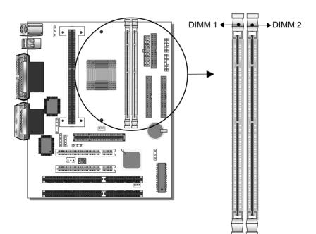
Your board comes with two DIMM sockets, providing support for up to 256MB of main memory using DIMM modules from 8MB to 128MB with no restriction on memory configuration. Therefore, you can install memory modules in any combination.
