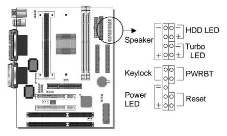
Plug the computer case's front panel devices to the corresponding headers on the mainboard.
