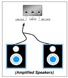
*Note:* This mainboard requires a speaker with **built-in amplifier** (Amplified Speaker) to generate proper output sound volume.
