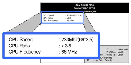
Available [CPU Speed] settings on your SY-6IEM Mainboard are detailed in the following table. If you set this field to [Manual], you are then required to fill in the next two consecutive fields: (1) the CPU Ratio, and (2) the CPU Frequency.
