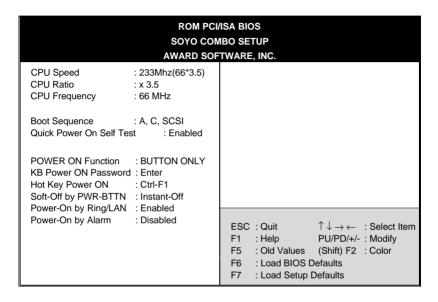
After the hardware installation is complete, turn the power switch on, then press the <DEL> key during the system diagnostic checks to enter the Award BIOS Setup program. The CMOS SETUP UTILITY will display on screen. Then, select the [SOYO COMBO SETUP] option from the main menu and press the <Enter> key.
