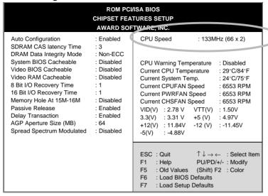
The 133/200MHz setting is used as default so whenever the BIOS settings are erased or reset the board will be able to boot up. However, there is no Pentium<sup>®</sup> II processor of that frequency.
