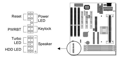
Plug the computer case's front panel devices to the corresponding connectors on the motherboard.
