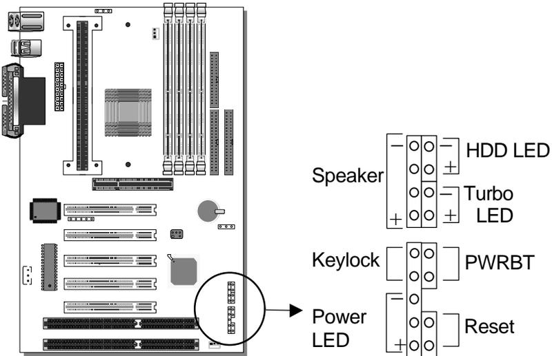
Plug the computer case's front panel devices to the corresponding headers on the mainboard.
