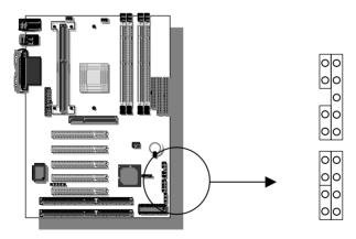
Plug the computer case's front panel devices to the corresponding connectors on the motherboard.
