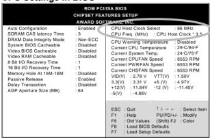
The 133/200MHz setting is used as default so whenever the BIOS settings are erased or reset the board will be able to boot up. However, there is no Pentium<sup>®</sup>II processor of that frequency.
