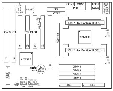
Figure 1–2. Mainboard Default Setting
