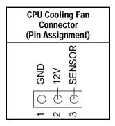
Note: Make sure the pin assignment of our CPU Cooling Fan is matched with this connector before connecting it, otherwise, you may damage either the mainboard or the cooling fan.
