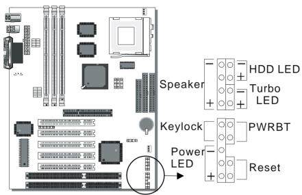
Plug the computer case's front panel devices to the corresponding connectors on the Motherboard.
